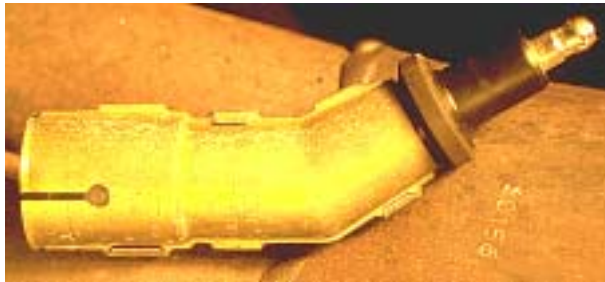
The spark plug shroud. This should pull off but it can be quite stubborn. In the background is the exhaust manifold.
