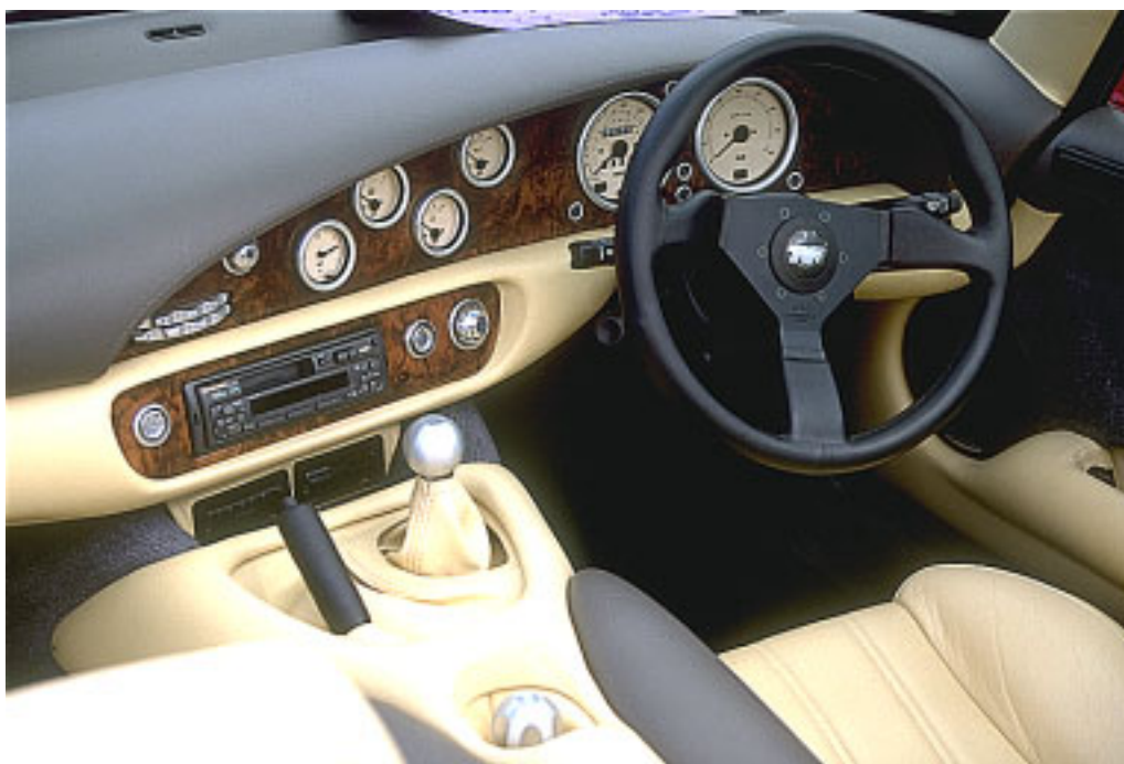
1995 Chimaera with coloured instruments. Note the rev limit band on the rev counter and the fluted door opening knob in the centre of the transmission.
